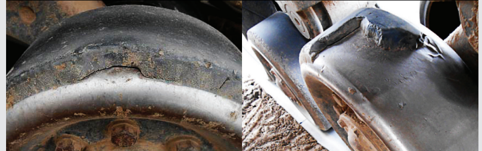
Major damage to outer surface and significant separation from the metal hubs.
